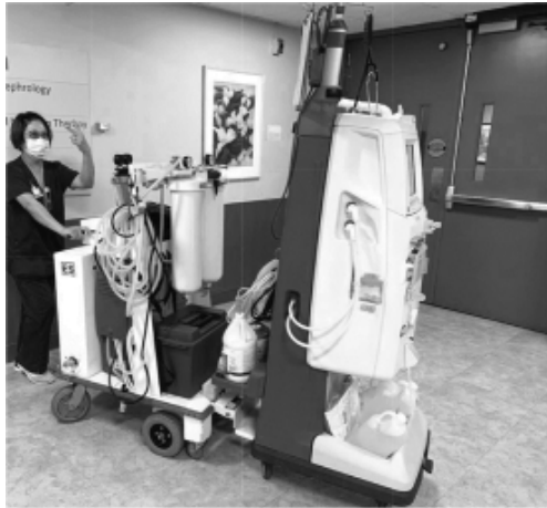
Traditional Hemodialysis Machine with Water Filtration Equipment
