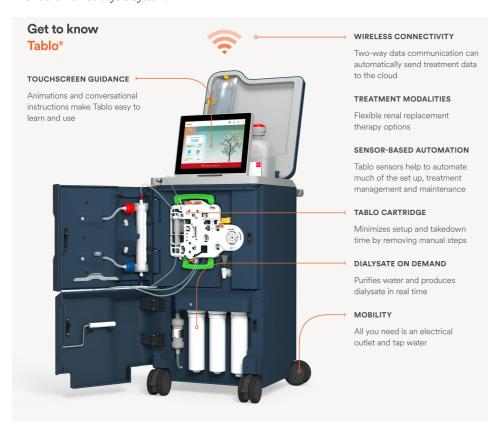
Tablo is the only dialysis technology with a fully integrated water treatment system that allows for dialysate to be produced on demand in real time using bicarbonate and acid concentrates. The Tablo console requires only a standard electrical outlet and tap water to operate. This eliminates the need for industrial water treatment rooms, separate water purification machines and pre-filled bags of dialysate associated with traditional dialysis machines.
