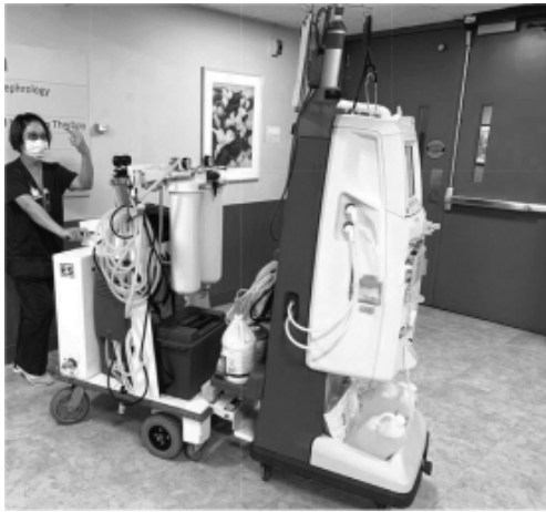
Traditional Hemodialysis Machine with Water Filtration Equipment
