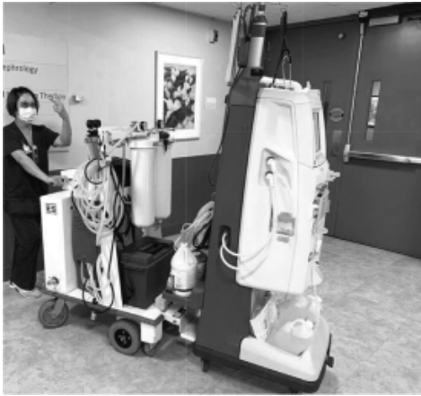
Traditional Hemodialysis Machine with Water Filtration Equipment
